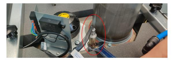
2. Screw on spacer at the end of the lambda sensor
