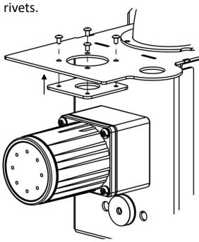
**5.** Secure your new 12 pin motor print to the burner.
